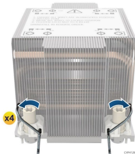
Figure 85. Processor Heat Sink Anti-tilt Wires in the Outward Position
