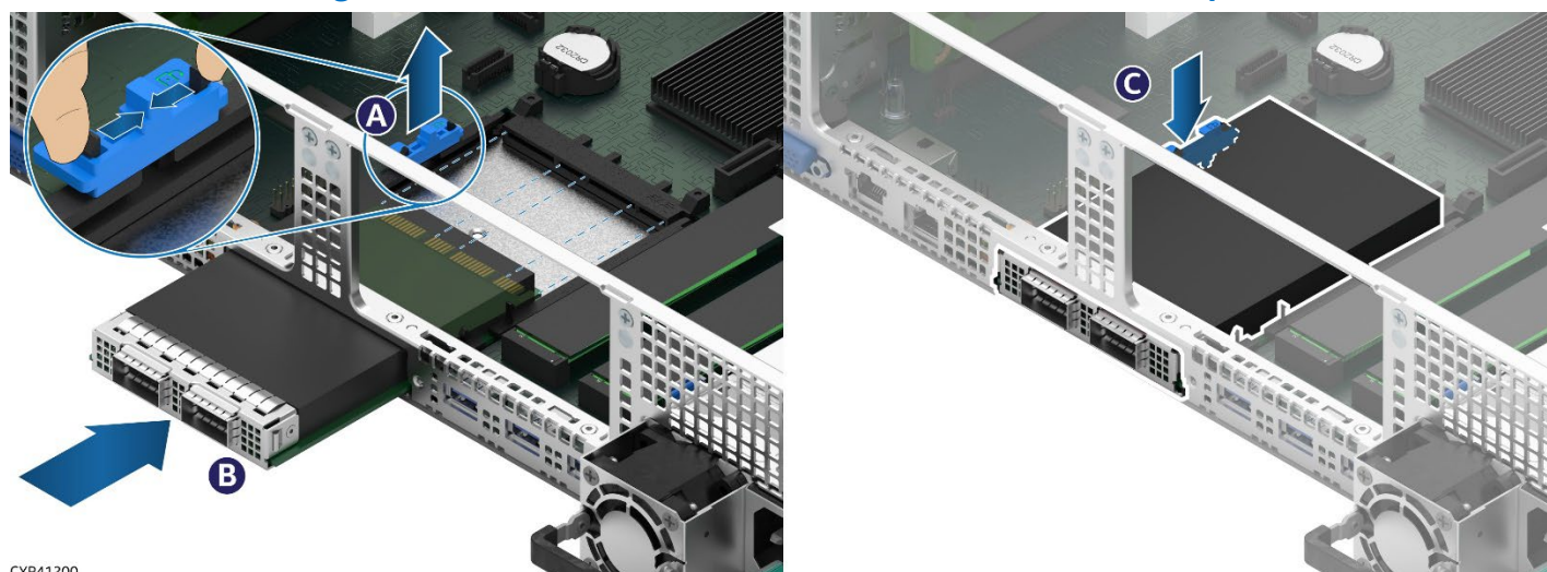
Figure 63. OCP 3.0 Add-in Card Installation – Internal Lock Option
