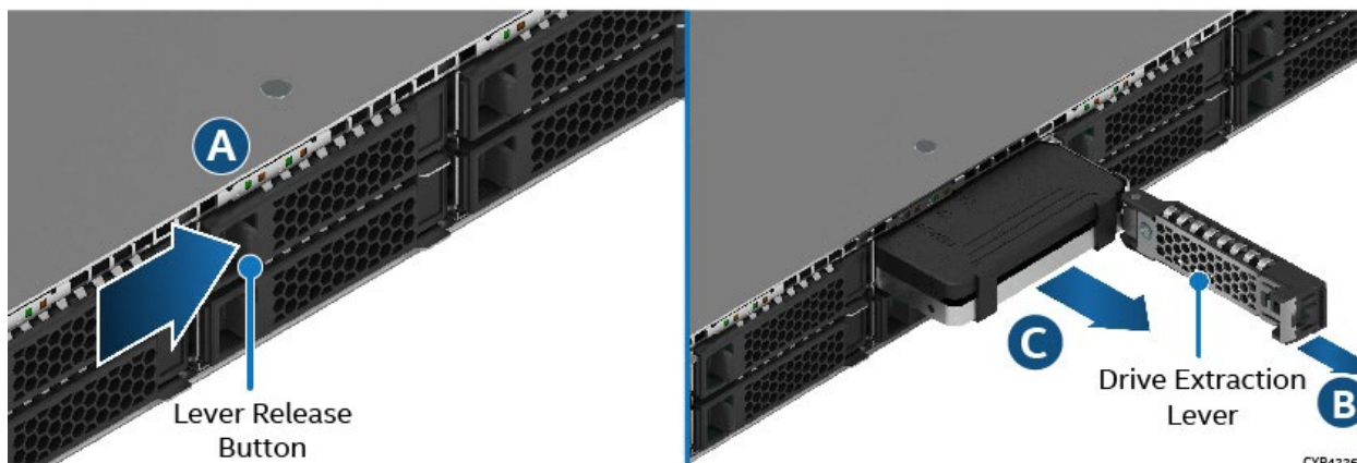
Figure 51. Drive Removal from Drive Bay
