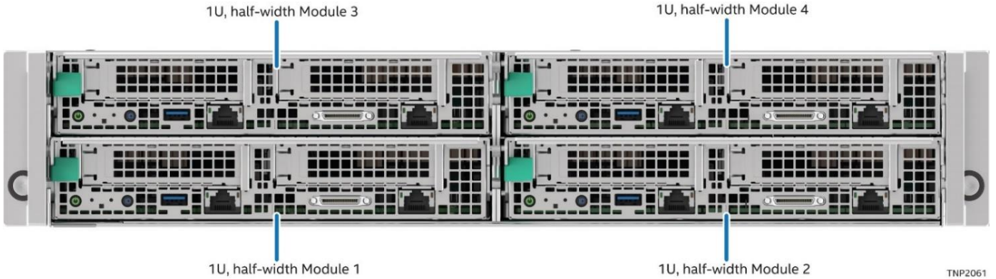
Figure 40. Module Identification for Four-Module System Configuration
