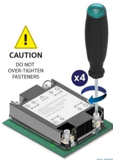
Figure 141. Tighten Heat Sink Fasteners
