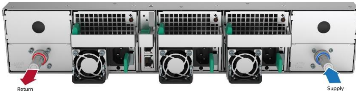
Figure 85. Chassis Plumbing Couplings Identification
