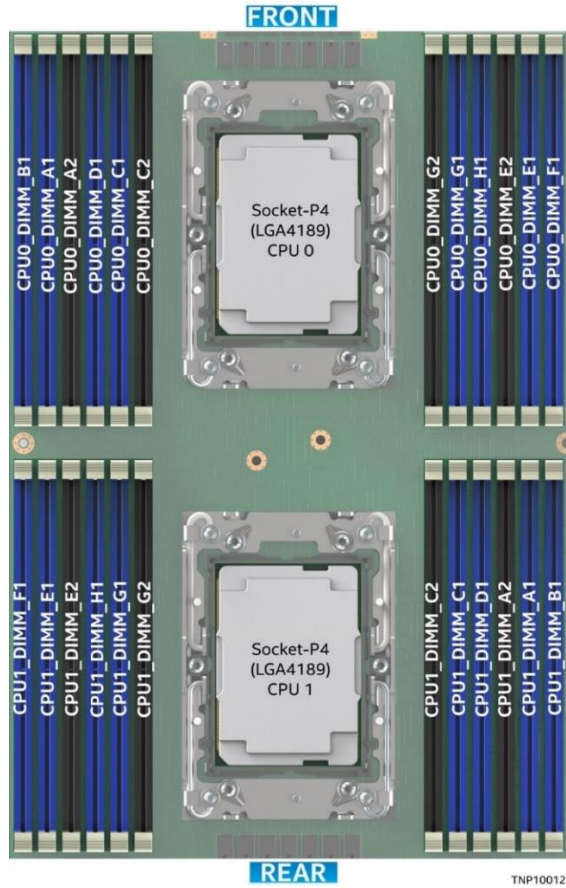
Figure 58. Intel® Server Board D50TNP1SB Memory Slot Layout
